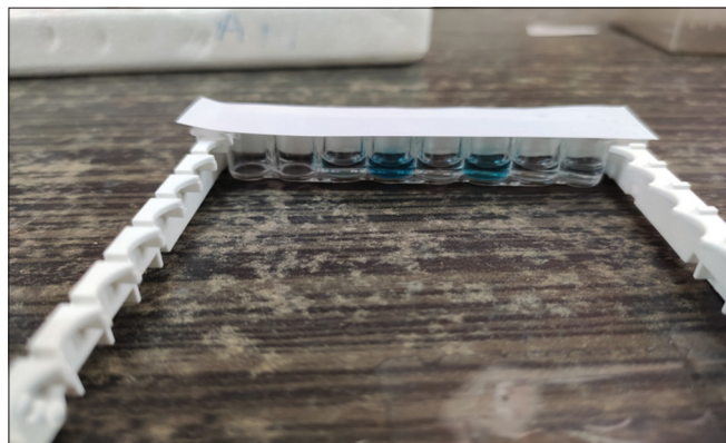
Figure 4: Well of ELISA strip showing the blue color on dengue positive samples
