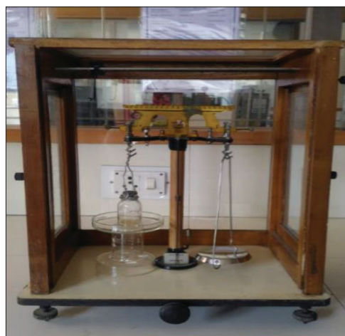
Figure 1: Measurement of mucoadhesive force of in situ gel
